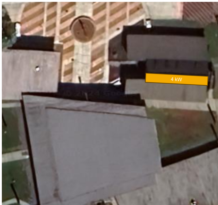
Figure 9. Potential housing rooftop solar PV. Existing skylights (covered by orange box) will reduce the amount of space available.
