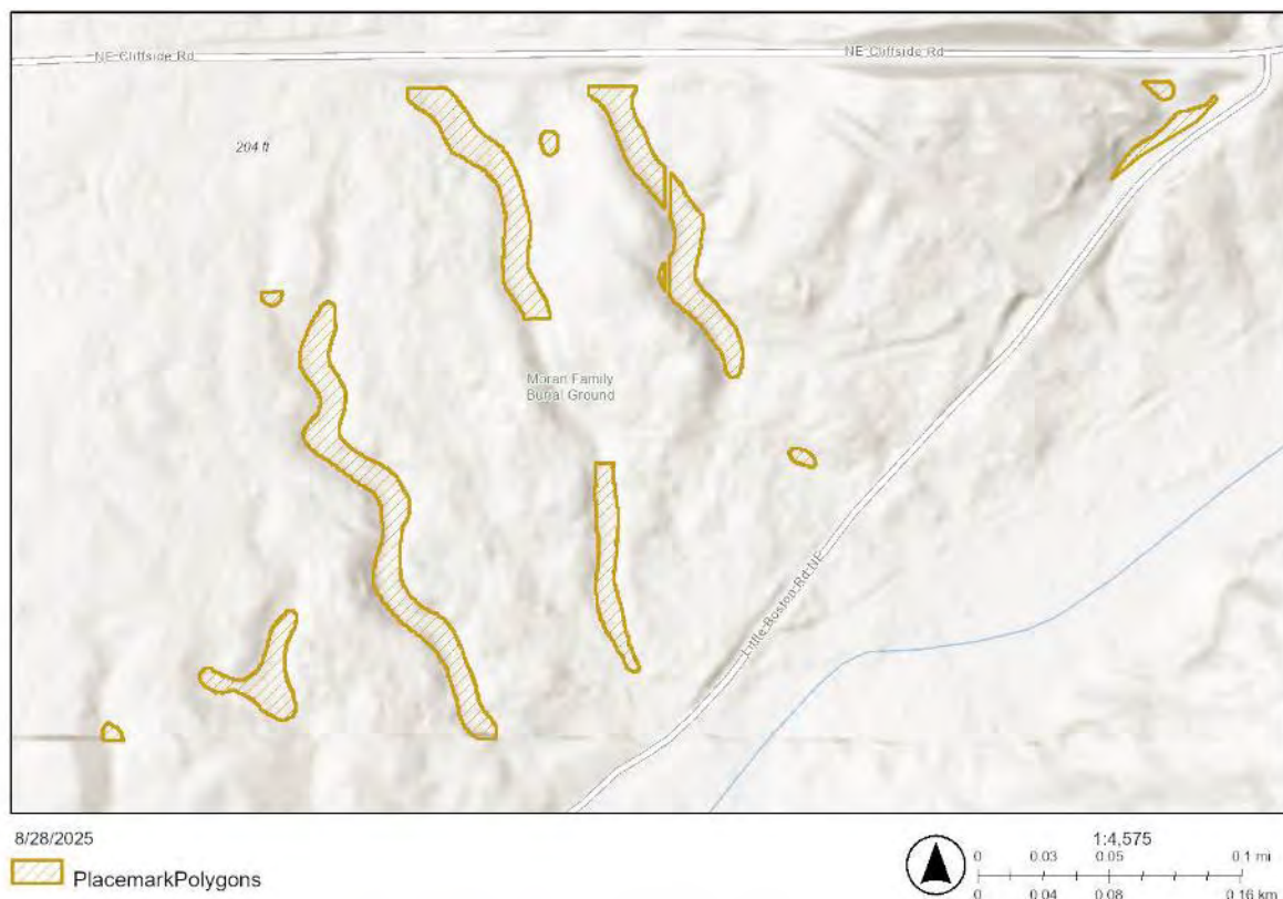
Figure 3. Potential wetland areas based on lidar low points in Hansville Block Site 2 (Source: PGST Natural Resources GIS)
